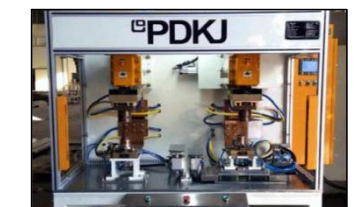
Automatic welding machine for car subframe
