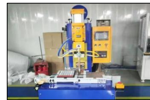
Customized copper precision parts automatic spot welding machine
