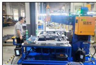
Galvanized plate chassis automatic spot welding machine
