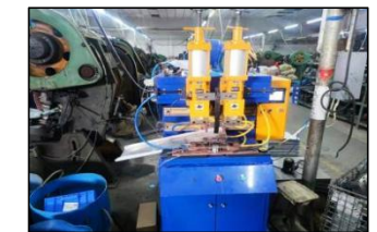
Double head automatic spot welding machine
