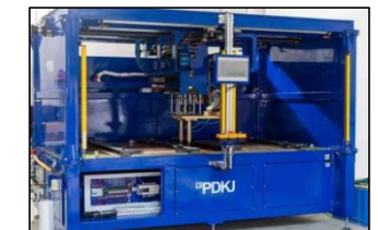
Double head reinforcing rib automatic spot welding machine
