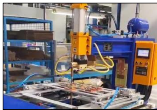
Customized electric heating wire automatic spot welding machine
