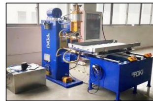
Customized XY axis chassis automatic spot welding machine
