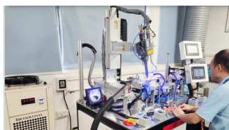
Application of multi axis galvanometer laser welding
