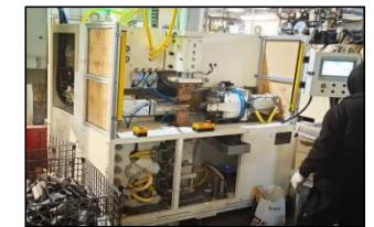
BYD customized double-sided car bracket spot welding machine
