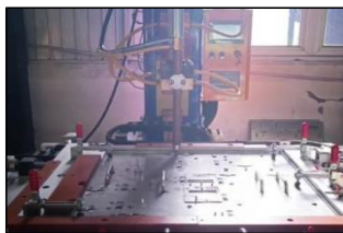
Xy axis chassis automatic spot welding machine
